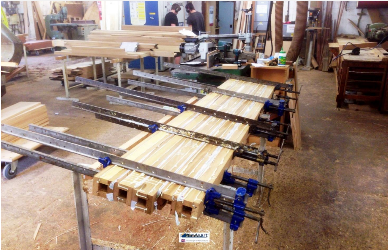
Terrafirma - glue laminated and clamped to the steel core - ShadeArt UK
