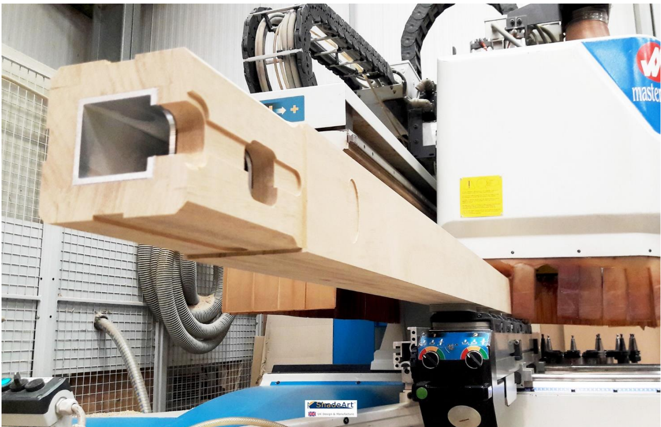
Terrafirma - CNC Milling Machined after glue lamination - ShadeArt UK
