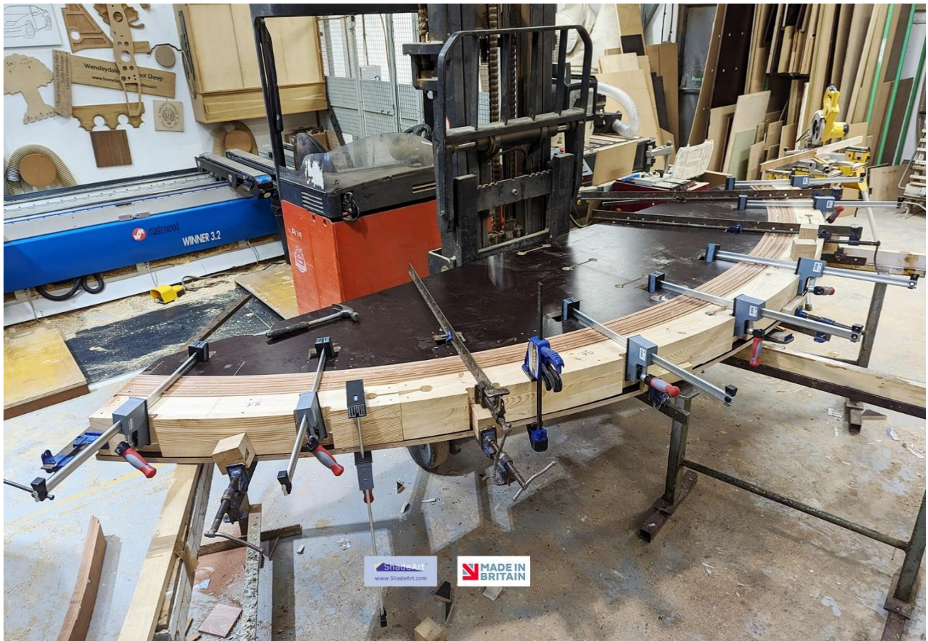
Terrafirma Arched - Held and glued in our Jig - ShadeArt UK
